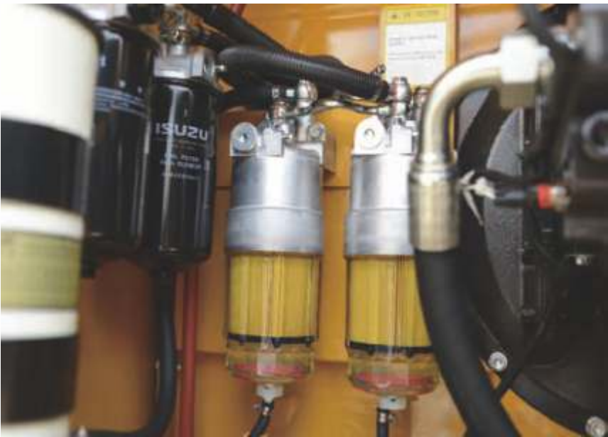
Large capacity multi-stage filtration system
