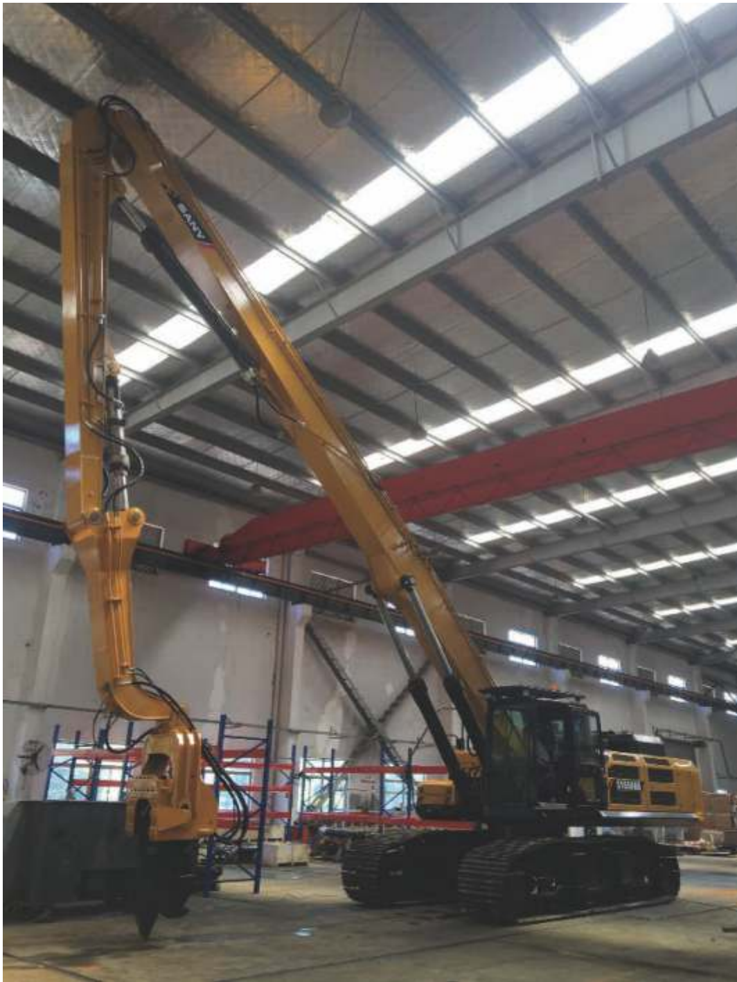
SY650HD is equipped with an 18 meter pile driving arm
