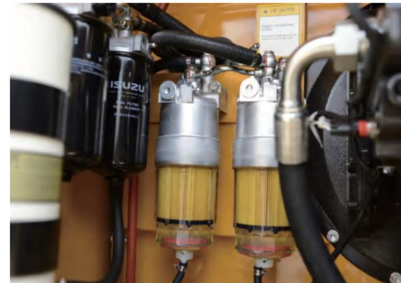
High-capacity multi-stage filter system
